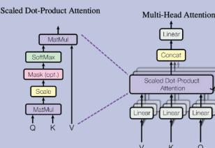
Multi-Head Attention consists of linear layers split into heads, followed by scaled dotproduct attention, oncatenation of heads and a final linear layer.
